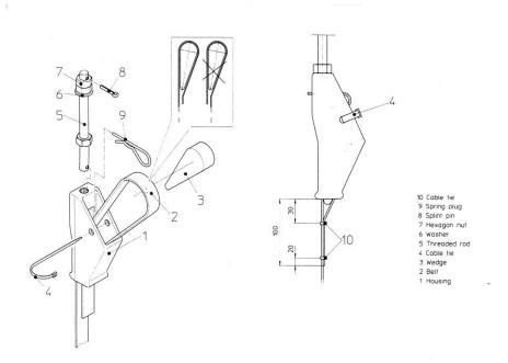
10. In order to prevent a possible pulling through of the belt while assembling or a possible loosening of the wedge while operating, the dead end side of the belt has to be secured. Upon securing the dead end side of the belt, different operating conditions have to be considered. Depending on these conditions, different methods are proposed for treatment of the non bearing end of the belt.
